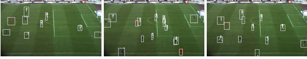
Figure 3: Frames of a soccer video dataset with detected and tracked objects using the DDPMO model in the probabilistic programming system Anglican.
